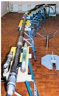
V.V. Karmazenko presenting in the workshop the production program of open hole modular logging strings for geophysical survey of oil and gas wells, 2006
