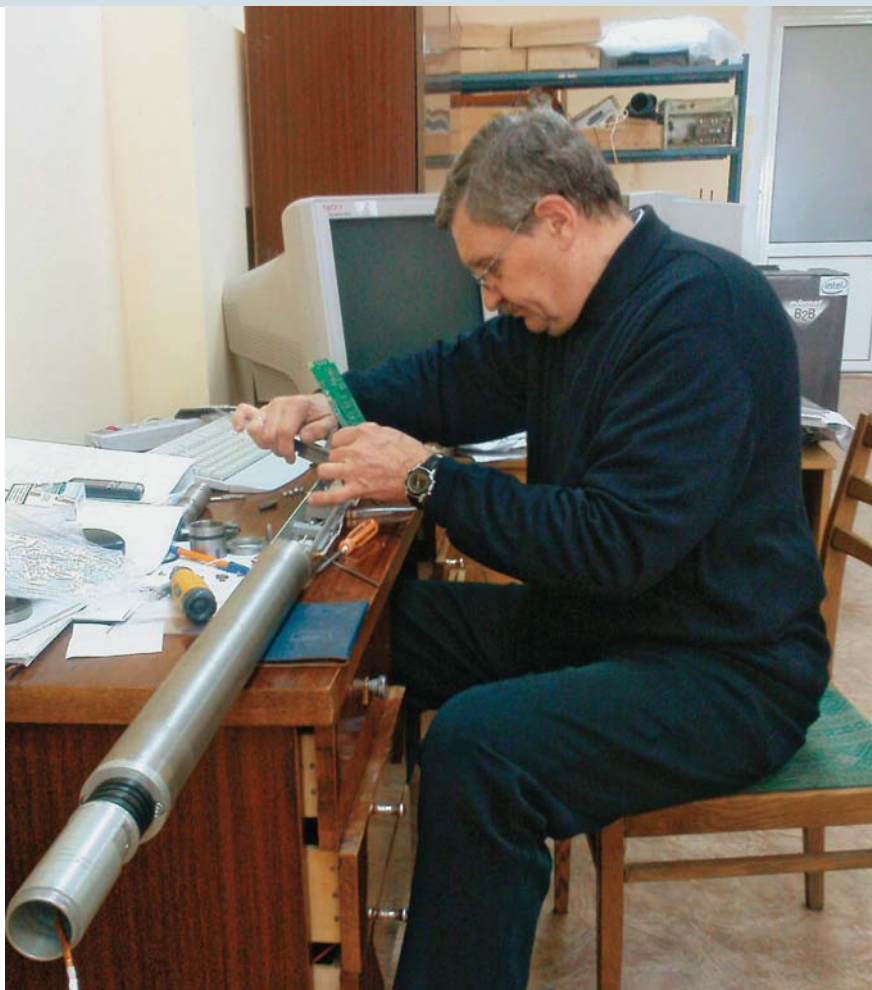
Glubokov, Anatoliy Oleksandrovych— Leading Expert in tool designing for radioactive logging, working on multi-probe neutron log tool
