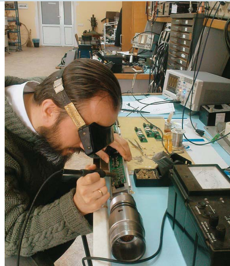
Zadorozhnyi, Sergiy— Engineer, testing the telemetry system of well geophysical equipment
