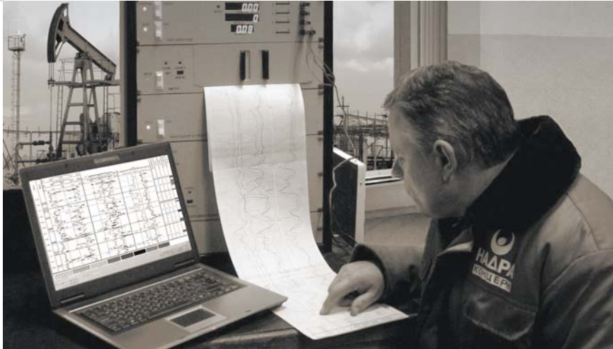
Digital registration of well logging data in production oil well
