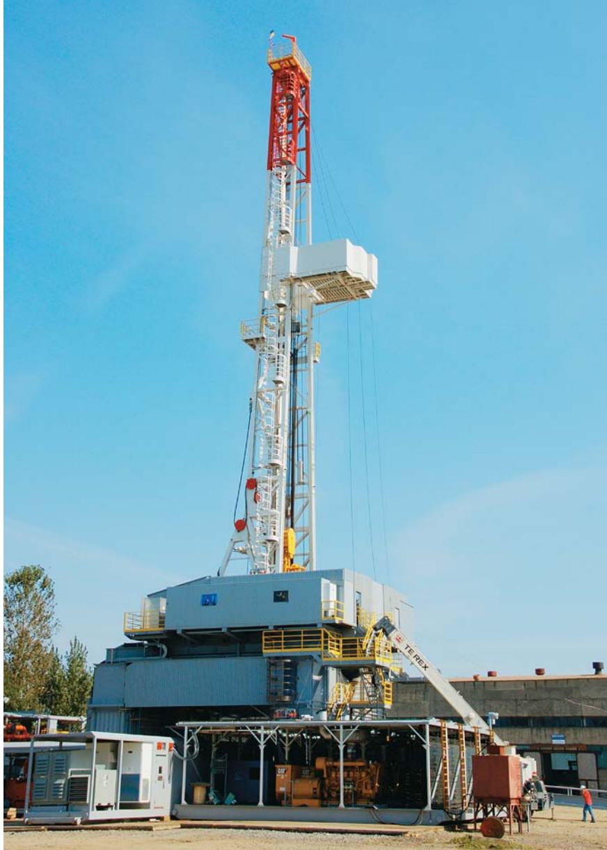
One of drilling rigs with load capacity of 600 t produced by the company on order of Weatherford
